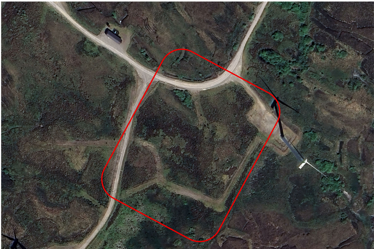
Photo 6 – Recent aerial photo of bunded peat repository cells on the Tullynahaw Wind Farm in Co. Roscommon.
